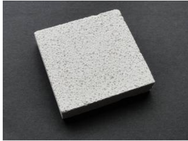
Figure 13: Sample of the highly insulating rendering. The pores are filled with transparent nanoporouse Aerogel
