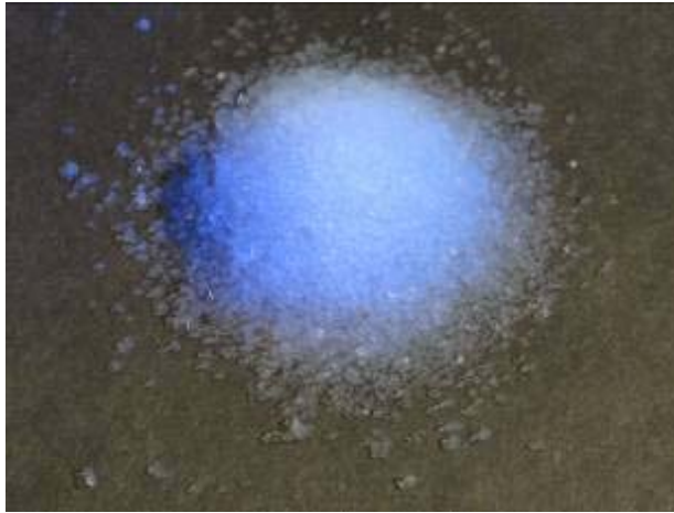
Figure 12: About 85% nanoporouse aerogel granulate is used as additive for the light weight plaster
