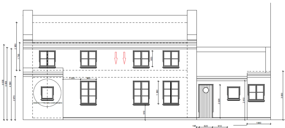
Figure 31- Red arrows indicating the position of the flux sensors.
