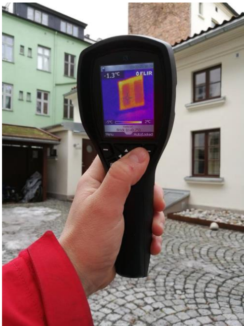
Figure 29- Using the FLIR I3 thermal imaging camera.
